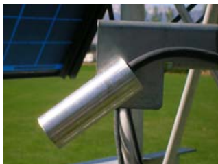
Accurate measurement of canopy temperature is required to determine canopy stomatal conductance ( g_c ).
