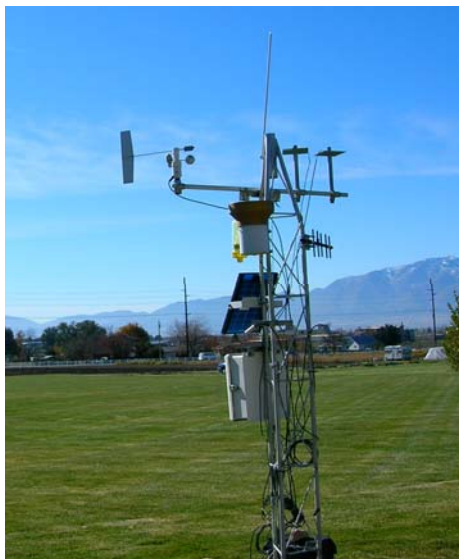
Canopy stomatal conductance ( g_c ) can be calculated by adding a measurement of canopy temperature to a standard ET station.
