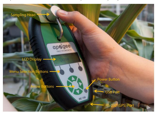
Press the power button to turn on the MC-100. After a few seconds the main menu screen appears. Program flow is organized into three menu groups. The selectable options are **Run** – used to set up and take measurements, **Data** – allows access and downloading of data files, and **System** – used to set up functional features of the meter and view system diagnostics.
