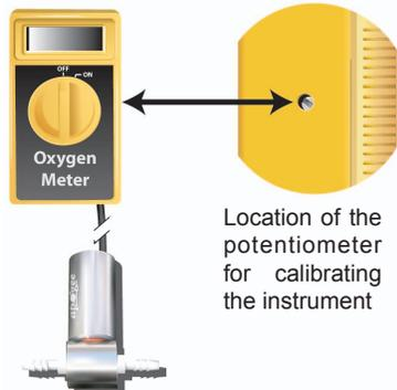
Location of the potentiometer for calibrating the instrument
