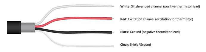
Wiring for ST-100 Serial Numbers range 0-2724, ST-110 Serial Numbers range 0-2724, and ST-200 Serial Numbers range 0-1351
