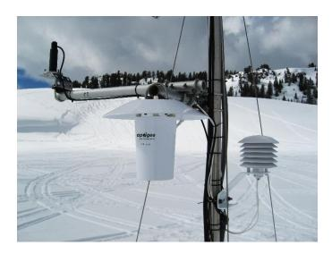
Top left: SP-230 Heated Pyranometer
