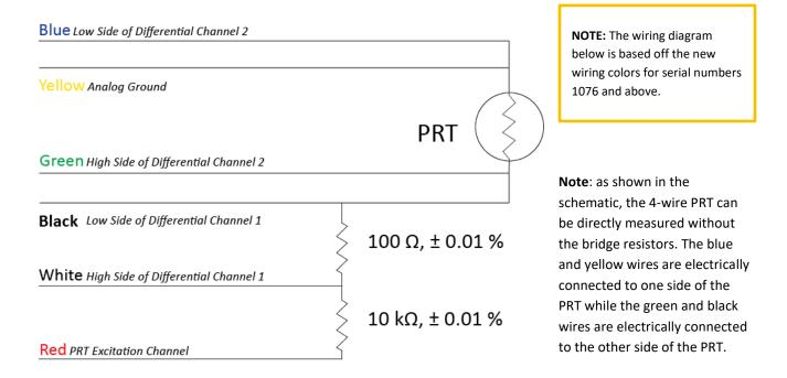
An excitation voltage of 2.1 V DC is recommended to minimize current drain, while still maintaining an adequate voltage signal. However, other excitation voltages can be used. Decreasing the excitation voltage will decrease current drain but will also decrease output voltage. Increasing the excitation voltage will increase output voltage but will also increase current drain.
