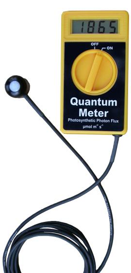
Our basic meter with a separate sensor to measure photosynthetically active radiation (PAR) in photon flux (PPF).
