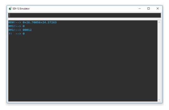
\*Note that the AC-421 automatically does the D0 command after a M1 is sent in order to display the results of the measurement.
