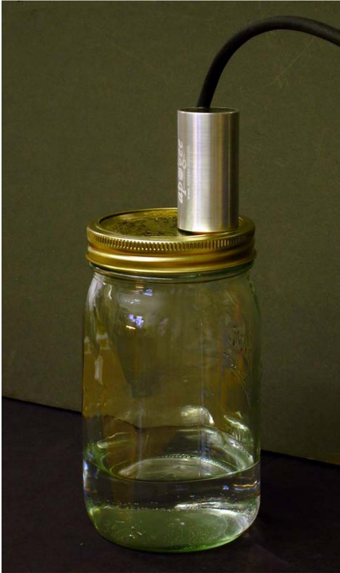
**Figure 4:** Apogee O<sub>2</sub> sensor mounted in a sealed chamber over water. For measurements in environments where the  $RH = 100\%$ , sensors should be calibrated in conditions where the  $RH = 100\%$  in order to account for any humidity effects on sensor electronics.
