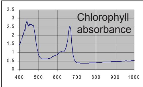
The CCM-200 uses absorbance to estimate the chlorophyll content in leaf tissue. Two wavelengths are used for absorbance determinations. One wavelength falls within the chlorophyll absorbance range while the other serves to compensate for mechanical differences such as tissue thickness. The meter measures the absorbance of both wavelengths and calculates a Chlorophyll Concentration Index (CCI) value that is proportional to the amount of chlorophyll in the sample.
