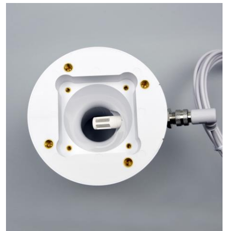
EE08 mounted inside TS-100 fan-aspirated radiation shield.
