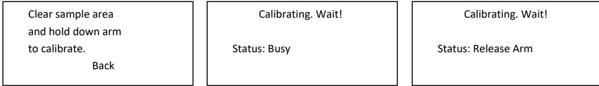
The MC-100 requires a calibration when taking the first measurement after powering on the unit. **Calibration is not required between measurements.** Verify the sample chamber’s optical path is clear and hold down the measuring arm until the **Release Arm** message is displayed.
