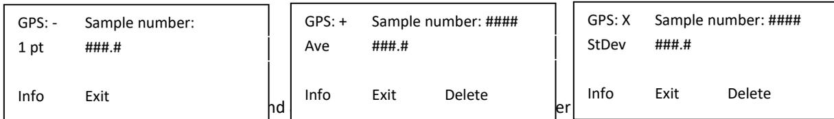
the status of the GPS signal and location logging ability. A “-” = GPS enable, no signal. A “+” = GPS enabled, signal acquired. An “X” = GPS disabled.
