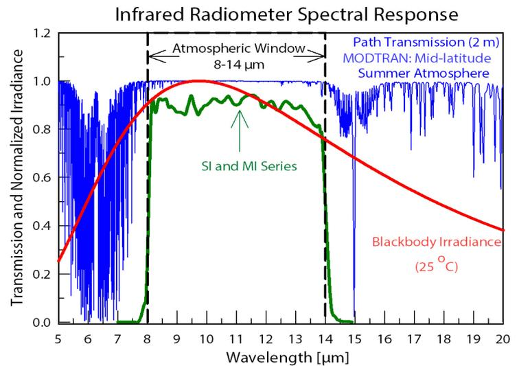
Above: Spectral response of SI series infrared radiometers. Spectral response (green line) is determined by the germanium filter and corresponds closely to the atmospheric window of 8 to 14 μm, minimizing interference from atmospheric absorption/emission bands (blue line) below 8 μm and above 14 μm. Typical terrestrial surfaces have temperatures that yield maximum radiation emission within the atmospheric window, as shown by the blackbody curve for a radiator at 25 C (red line).
