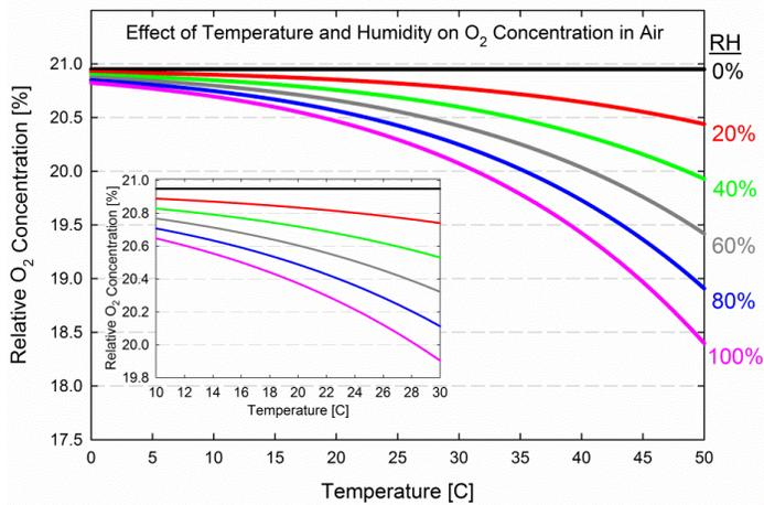
For measurements in soil or saturated air (100 % relative humidity), it is recommended that the MO-200 is calibrated in conditions where relative humidity is 100 %. A simple way to accomplish this is to mount the sensor in a sealed chamber over water, with ambient air filling the headspace, as shown below.
