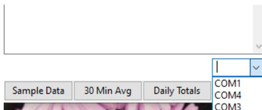
When you have connected to the correct COM#, the software will say “Connected”.
