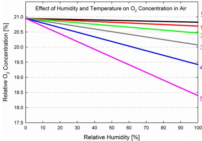
A) Relative humidity effects on relative oxygen concentration shown as a function of relative humidity at temperatures increments of 10 C and B) as a function of temperature at relative humidity increments of 20 %. The air in soil is typically always saturated with water vapor (100 % relative humidity) unless the soil is very dry.
