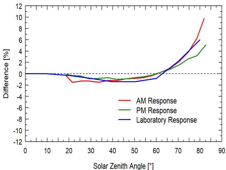
Mean directional (cosine) response of six apogee SQ-100 series quantum sensors. Directional response measurements were made on the rooftop of the Apogee building in Logan, Utah. Directional response was calculated as the relative difference of SQ-500 quantum sensors from the mean of replicate reference quantum sensors (LI-COR models LI-190 and LI-190R, Kipp & Zonen model PQS 1). Data were also collected in the laboratory using a reference lamp and positioning the sensor at varying angles.
