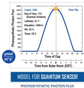
Homepage of the Clear Sky Calculator. Two calculators are available: one for quantum sensors (PPFD) and one for pyranometers (total shortwave radiation).
