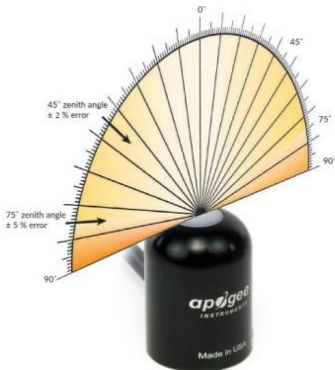
Directional (cosine) response is defined as the measurement error at a specific angle of radiation incidence. Error for Apogee SQ-100 series quantum sensors is approximately  $\pm 2\%$  and  $\pm 5\%$  at solar zenith angles of  $45^\circ$  and  $75^\circ$ , respectively.
