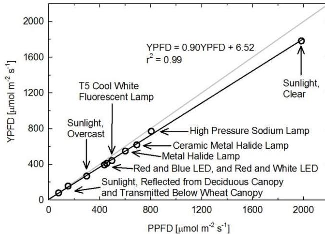
Correlation between photosynthetic photon flux density (PPFD) and yield photon flux density (YPFD) for multiple different radiation sources. YPFD is approximately 90 % of PPFD. Measurements were made with a spectroradiometer (Apogee Instruments model PS-200) and weighting factors shown in the previous figure were used to calculate PPFD and YPFD.
