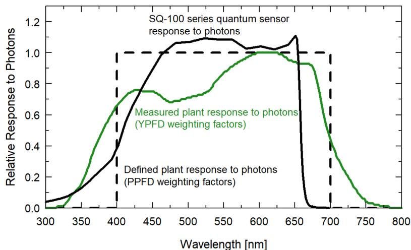
Defined plant response to photons (black line, weighting factors used to calculate PPFD), measured plant response to photons (green line, weighting factors used to calculate YPFD), and SQ-100 series and SQ-300 series quantum sensor response to photons (sensor spectral response).
