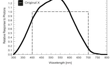
Mean **cosine response** of twenty-three SQ X series quantum sensors.
