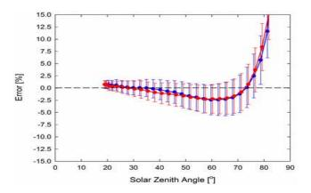
Mean **cosine response** of twenty-three MQ-210 quantum sensors (error bars represent two standard deviations above and below mean). Cosine response measurements were made by direct side-by-side comparison to the mean of four reference thermopile pyranometers, with solar zenith angle-dependent factors applied to convert total shortwave radiation to PPFD. Blue points represent the AM response and red points represent the PM response.
