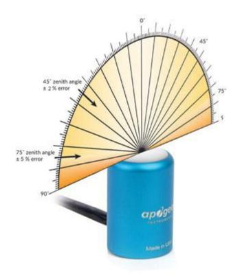
Directional (cosine) response is defined as the measurement error at a specific angle of radiation incidence. Error for Apogee MQ-500 series quantum sensors is approximately  $\pm$  2 % and  $\pm$  5 % at solar zenith angles of 45° and 75°, respectively.
