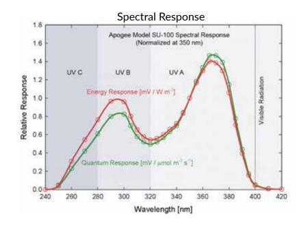
Spectral response estimate of Apogee SU-100 UV sensors. Spectral response measurements were made at 10 nm increments across a wavelength range of 200 to 450 nm in a monochromator with an attached electric light source. Measured spectral data were normalized at 350 nm.
