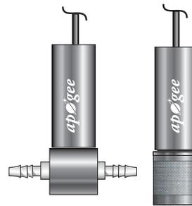
**For the most stable reading, the sensor should be used with the sensor opening facing down.** This facilitates the best contact of the electrolyte with the O<sub>2</sub> sensing elements.
