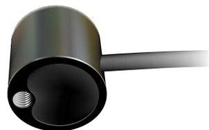
Each sensor is equipped with a mounting bolt. Mount the sensor as level as possible. Small changes in level can cause measurement errors. We recommend using our leveling plate (model LEV) for the most accurate measurements. The sensor should be mounted with the cable pointing toward the nearest magnetic pole to minimize azimuth error.
