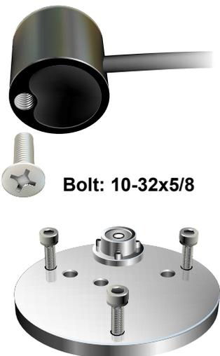
Each sensor is equipped with a mounting bolt. Mount the sensor as level as possible. Small changes in level can cause measurement errors. We recommend using our leveling plate (model LEV) for the most accurate measurements. The sensor should be mounted with the cable pointing toward the nearest magnetic pole to minimize azimuth error.
