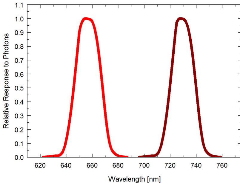
Mean spectral response measurements of six replicate red - far-red sensors (red sensor is centered near 655 nm, far-red sensor is centered near 730 nm). Spectral response measurements were made at 2 nm increments across a wavelength range of 600 to 800 nm in a monochromator with an attached electric light source. Measured spectral data from each sensor were normalized by the measured spectral response of the monochromator/electric light combination, which was measured with a spectroradiometer.
