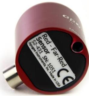
A sensor's model number and serial number are located on the bottom of the sensor. If you need the manufacturing date of your sensor, please contact Apogee Instruments with the serial number of your sensor.
