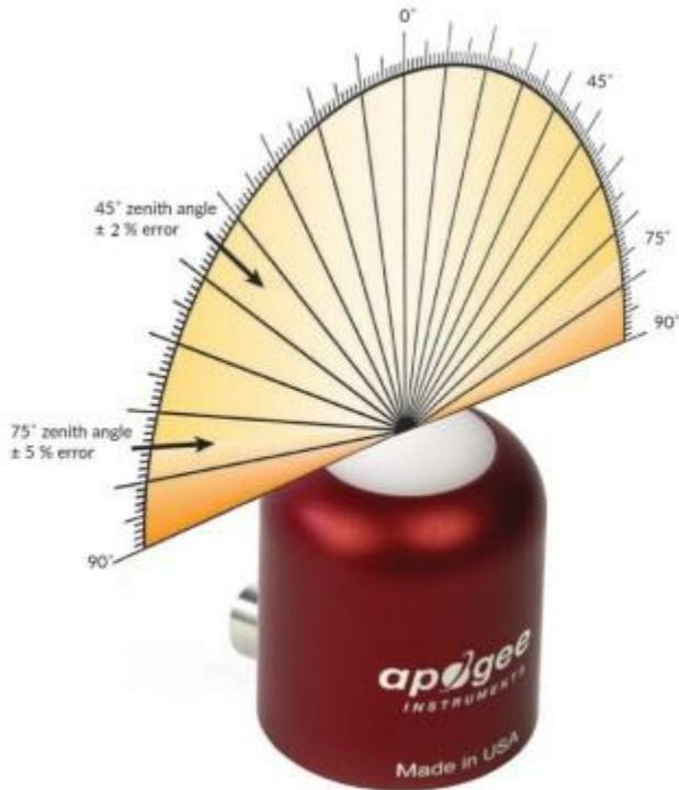
Directional, or cosine, response is defined as the measurement error at a specific angle of radiation incidence. Directional error for Apogee S2 series red - far-red sensors is approximately ± 2 % and ± 5 % at solar zenith angles of 45° and 75°, respectively.
