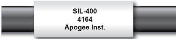
A sensor's model and serial numbers are located on a label near the pigtail leads on the sensor cable. If you need the manufacturing date of your sensor, please contact Apogee Instruments with the serial number of your sensor.
