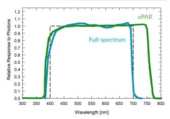
Spectral response of the SM-500 PAR sensor (blue) and SM-600 ePAR sensor (green) compared to the traditional PAR response (dashed).
