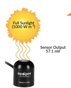
Example of total shortwave radiation measurement with an Apogee SP-510 pyranometer. Full sunlight yields total shortwave radiation on a horizontal plane at the Earth's surface of approximately 1000 W m<sup>-2</sup>. This yields an output signal of 57.1 mV (varies from sensor to sensor). The signal is converted to shortwave radiation by multiplying by the calibration factor of 17.5 W m<sup>-2</sup> per mv (approximately, varies from sensor to sensor)
