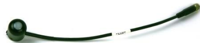
When sending sensors in for calibration, only send the short end of the cable and half the connector.
