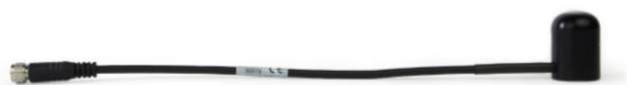
When sending sensors in for calibration, only send the short end of the cable and half the connector.
