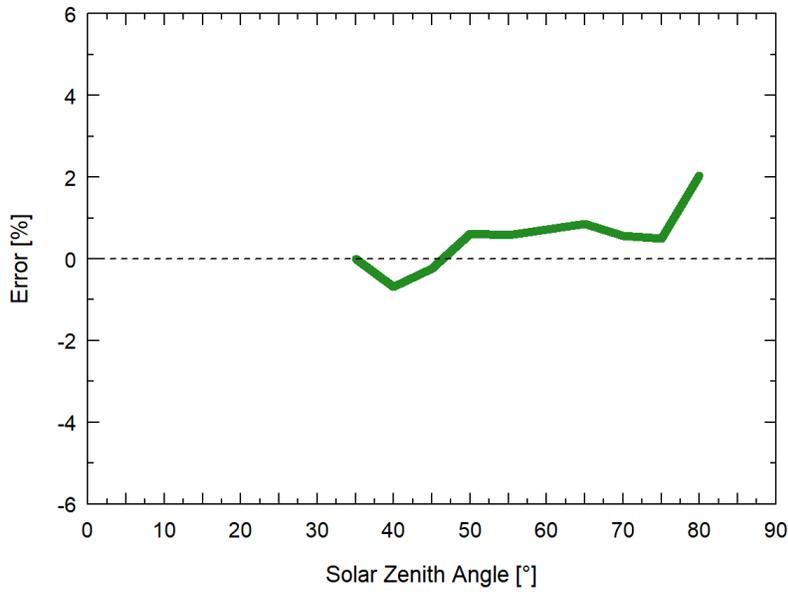
Mean cosine response of five SQ-100X series quantum sensors. Cosine response measurements were made by direct side-by-side comparison to the mean of seven reference SQ-500 quantum sensors.
