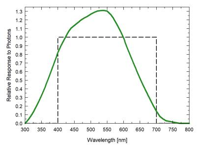
Mean spectral response of four SQ-100x series quantum sensors compared to PPFD weighting function. Spectral response measurements were made at 10 nm increments across a wavelength range of 350 to 800 nm in a monochromator with an attached electric light source. Measured spectral data from each quantum sensor were normalized by the measured spectral response of the monochromator/electric light combination, which was measured with a spectroradiometer.
