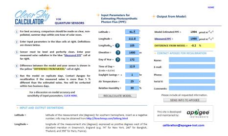
Clear Sky Calculator for quantum sensors. Site data are input in blue cells in middle of page and an estimate of PPFD is returned on right-hand side of page.
