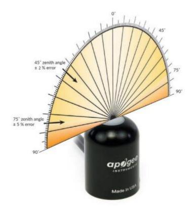
Directional, or cosine, response is defined as the measurement error at a specific angle of radiation incidence. Error for Apogee SQ-100X series quantum sensors is approximately  $\pm$  2 % and  $\pm$  5 % at solar zenith angles of 45° and 75°, respectively.
