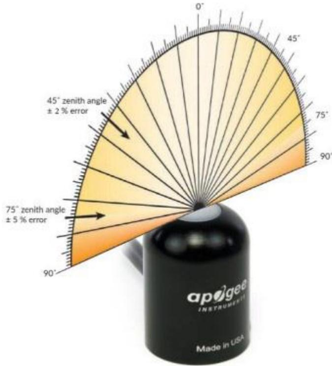
Directional, or cosine, response is defined as the measurement error at a specific angle of radiation incidence. Error for Apogee SQ-100X series quantum sensors is approximately ± 2 % and ± 5 % at solar zenith angles of 45° and 75°, respectively.
