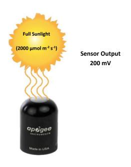
Example of PPFD measurement with an Apogee quantum sensor. Full sunlight yields a PPFD on a horizontal plane at the Earth's surface of approximately 2000  $\mu$ mol m<sup>-2</sup> s<sup>-1</sup>. This yields an output signal of 200 mV. The signal is converted to PPFD by multiplying by the calibration factor of 10.00  $\mu$ mol m<sup>-2</sup> s<sup>-1</sup> per mV.
