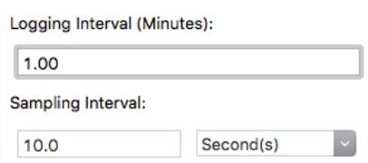
Before clicking ‘Get Logged Data’ it is important to set the time of the last logged data point. This is used to back calculate the timestamps for the remaining data points. If you just unplugged the sensor and plugged it into the computer the preloaded day and time should be sufficient.
