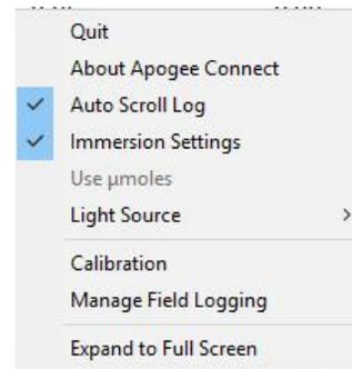
Clicking **'Calibration'** will display the factory calibrated multiplier and offset values. These values are saved in firmware and can be recovered by clicking the **'Recover Original'** button. Deriving a new calibration multiplier and offset is accomplished by clicking the **'Recalibrate'** button. This is applicable if users want to calibrate the sensor to their own specific light source. Note that a reference PFD value of the light source is required to complete a recalibration.
