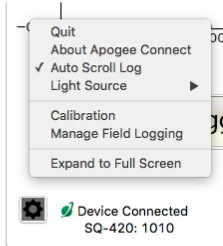
Note the **'Light Source'** function is not necessary for the SQ-626. The SQ-626 is calibrated for use under LED light sources; therefore, this function is not necessary for the SQ-626. The function is designed to give increased accuracy for the SQ-420.
