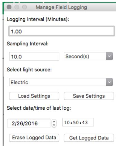
Set the sampling interval in minutes or seconds. The sampling interval is how often a measurement is taken and logging interval is how often the data is saved. The logged data is the average of the samples. The logging interval must be evenly divided by the sampling interval. For example if the logging interval is 5 minutes and the sampling interval is 2 minutes it causes an error. But a sampling interval of 1 minute is acceptable.
