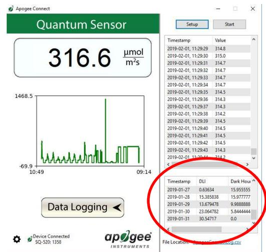
To use additional SQ-626 devices, open additional SQ-626 software windows. The device serial number will display in the lower left hand corner of the corresponding software window. Devices may be selected by serial number in the tool bar.
