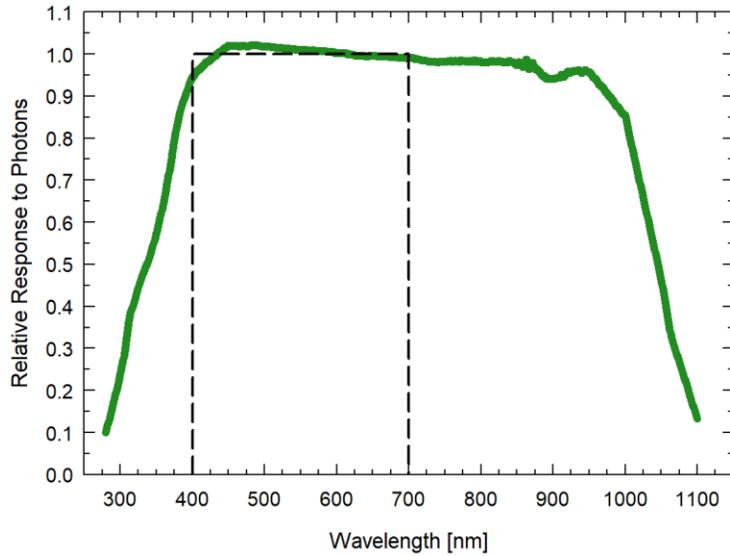
Mean spectral response measurements of six replicate Apogee SQ-600 series Extended Range PFD Sensors. Spectral response measurements were made at 10 nm increments across a wavelength range of 300 to 1100 nm in a monochromator with an attached electric light source. Measured spectral data from each PFD sensor were normalized by the measured spectral response of the monochromator/electric light combination, which was measured with a spectroradiometer
