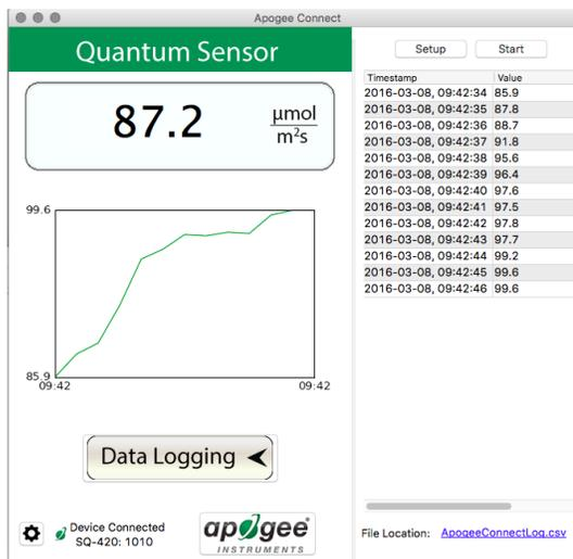
The data logging window can be closed without affecting logged data by clicking the 'Exit' button. The 'Stop' button must be clicked to end data logging.
