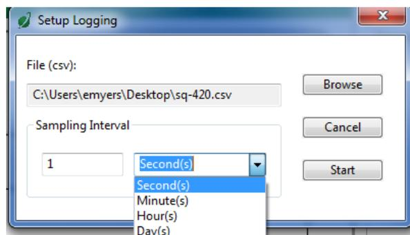
The data logging window will start to update at the specified sampling interval and display the Timestamp, Light Source, and Data Value. At the same time, data will be written to the csv file. Note that if the csv file is open in another program new data will not be saved to it.
