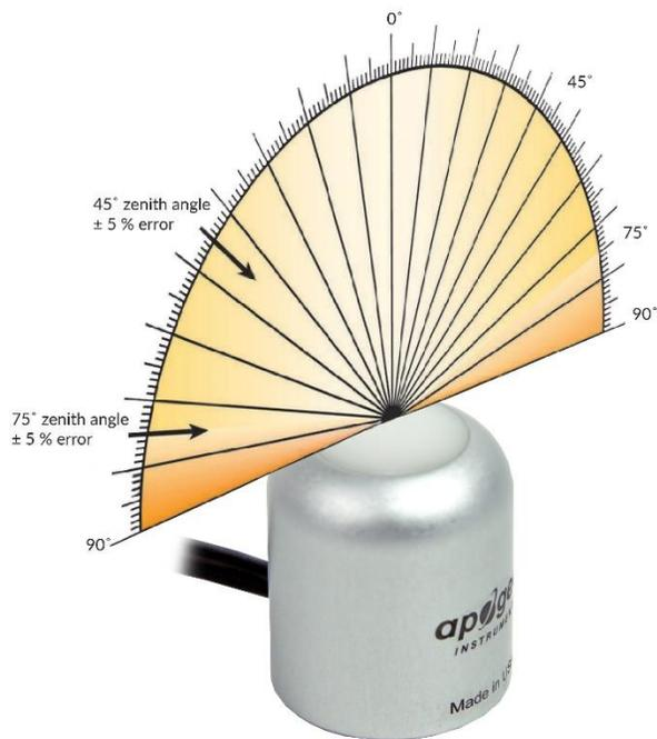
Directional, or cosine, response is defined as the measurement error at a specific angle of radiation incidence. Error for Apogee SQ-600 series Extended Range PFD Sensor is approximately  $\pm 2\%$  and  $\pm 5\%$  at solar zenith angles of  $45^\circ$  and  $75^\circ$ , respectively.
