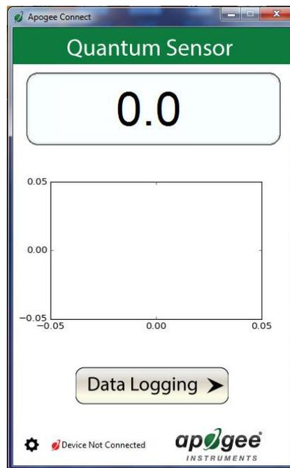
Plug the sensor into a USB port and allow some time for the sensor to automatically establish communication with the software. Once established, the message in the lower left corner will display "Device Connected-Model: SN ####" and real-time PFD readings will update on the screen. Moving the sensor closer to a light source should increase the readings, while blocking all light from the sensor should drop the reading to zero.
