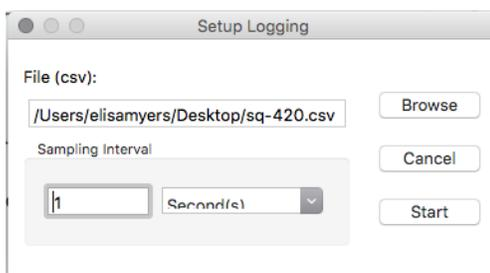
Select the desired sampling interval. Note that 1 second is the minimum interval allowed. Click 'Start'.
