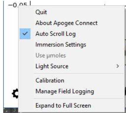
Note **'Light Source'** is not a selectable option. The SQ-626 is calibrated for use under LED light sources; therefore, this function is not necessary for the SQ-626. The function is designed to give increased accuracy for the SQ-420.
