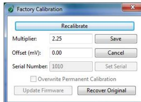
After clicking the 'Recalibrate' button the user will be prompted to cover the sensor. Place a dark cap over the sensor and wait for the real-time PFD reading to settle at zero. Click OK.
