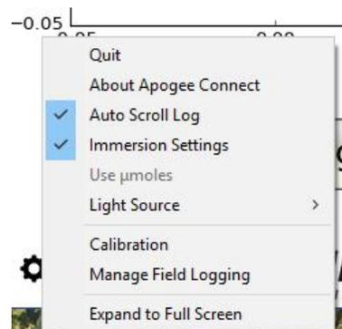
Clicking '**Calibration**' will display the factory calibrated multiplier and offset values. These values are saved in firmware and can be recovered by clicking the 'Recover Original' button. Deriving a new calibration multiplier and offset is accomplished by clicking the 'Recalibrate' button. This is applicable if users want to calibrate the sensor to their own specific light source. Note that a reference PFD value of the light source is required to complete a recalibration.
