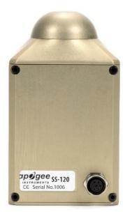
A sensor's model number and serial number are located on the back of the sensor.
