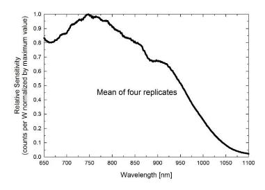
Sensitivity was determined by collecting spectra under a quartz halogen lamp with an NIST traceable calibration and calculating the ratio of counts measured with the spectrometer to energy flux density from the lamp. Maximum sensitivity of the SS-120 is near 750 nm. Sensitivity of the SS-120 is at least 10 % of the maximum value at all wavelengths less than 1030 nm.
