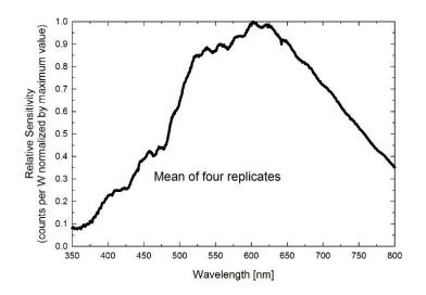
Sensitivity was determined by collecting spectra under a quartz halogen lamp with an NIST traceable calibration and calculating the ratio of counts measured with the spectrometer to energy flux density from the lamp. Maximum sensitivity of the SS-110 is near 600 nm. Sensitivity of the SS-110 is at least 10 % of the maximum value at all wavelengths greater than 380 nm.
