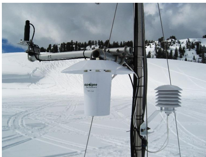
Top left: SP-230 Heated Pyranometer Center: TS-100 Fan Aspirated Radiation Shield Right: RM Young 41303 Static Solar Radiation Shield.
