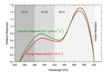
Spectral response estimate of Apogee SU-100 UV sensors. Spectral response measurements were made at 10 nm increments across a wavelength range of 200 to 450 nm in a monochromator with an attached electric light source. Measured spectral data were normalized at 350 nm.
