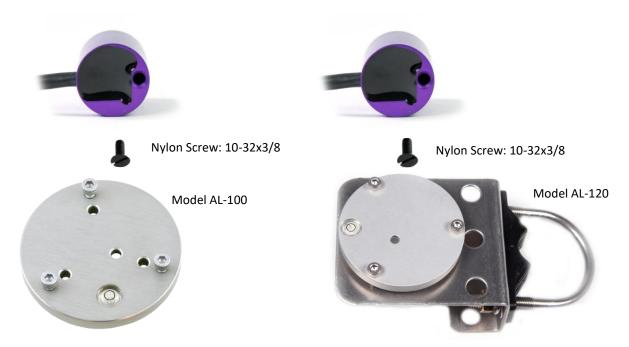
To minimize azimuth error, the sensor should be mounted with the cable pointing toward true north in the northern hemisphere or true south in the southern hemisphere. Azimuth error is typically less than 1 %, but it is easy to minimize by proper cable orientation.
