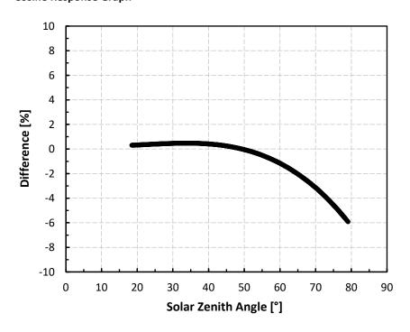
Mean cosine response of four Apogee UV-A sensors. Cosine response was calculated as the relative difference of UV-A sensors from the mean of replicate reference UV-A sensors deployed outdoors. These data are the average of the AM and PM response.
