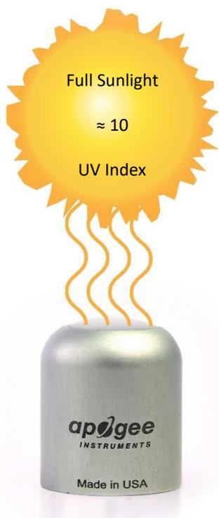
Example of UV Index and UV-B measurement with an Apogee UV-I/UV-B sensor. Full sunlight yields UV Index on a horizontal plane at the Earth's surface of approximately 10. This yields an output signal of 1 mV. The signal is converted to UV Index by multiplying by the calibration factor of 10 UV Index units per mV.
