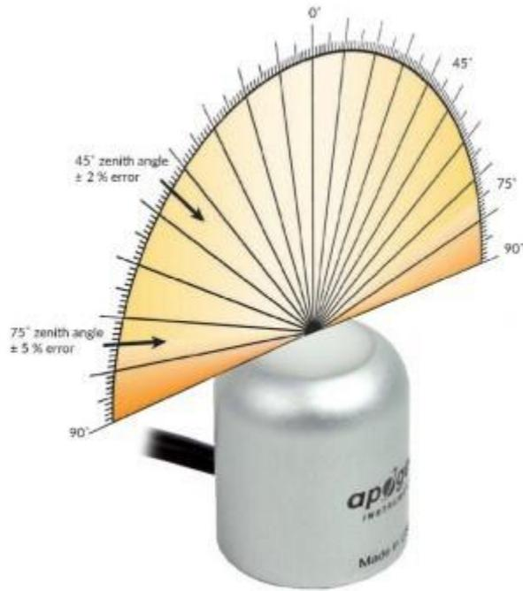
Directional, or cosine, response is defined as the measurement error at a specific angle of radiation incidence. Directional error for Apogee SU-300 series UV-I/UV-B sensors is approximately  $\pm 2\%$  and  $\pm 5\%$  at solar zenith angles of  $45^\circ$  and  $75^\circ$ , respectively.
