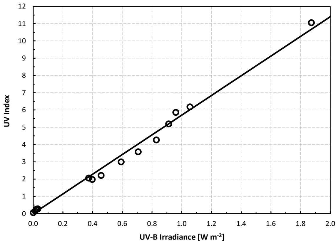
Relationship between UV Index and UV-B irradiance (in units of  $\text{W m}^{-2}$ ). Data are from multiple solar spectra representing a wide range of atmospheric conditions. Slope of the line is 5.7, with an  $r^2 = 0.99$ .
