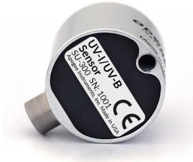
The model number and serial number are located on the bottom of the sensor. If manufacturing date of a sensor is required, please contact Apogee Instruments with the serial number of the sensor.
