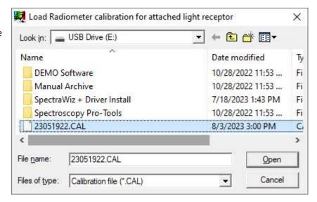
To confirm that calibration files have been loaded successfully there will be an sw.ini and an SW1.icf file located in the StellarNet folder found on the hard drive at C:\Program Files\StellarNet\SpectraWiz.
