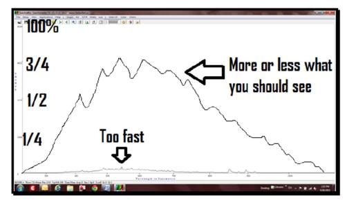
i. To adjust integration time, you can use the clock icon or click **Setup > Detector integration time.**
