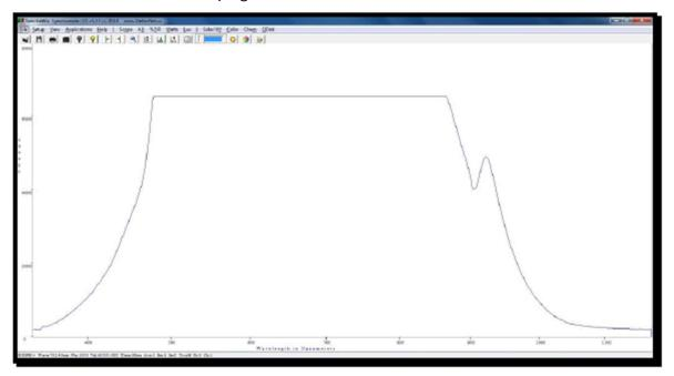
The above picture is of a saturated curve.
