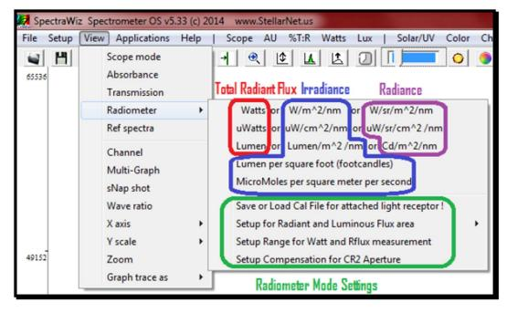
11c. The calibration type dictates if the measurement is Total Radiant Flux, Irradiance or Radiance.
