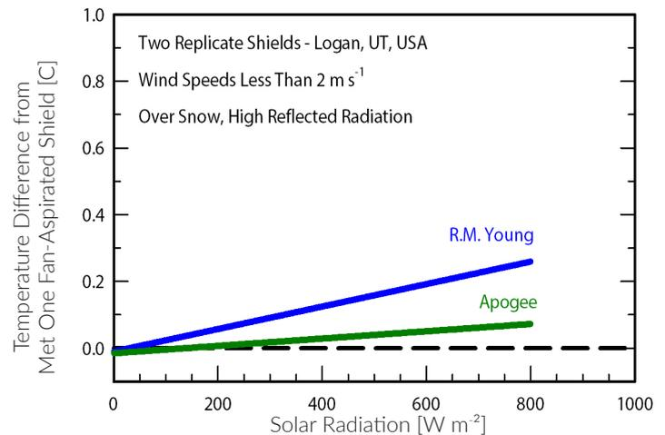
The performance of Apogee (model TS-100) and R.M. Young (model 43502) fan-aspirated shields relative to a Met One (model 076B) fan-aspirated shield.
