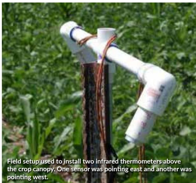
Field setup used to install two infrared thermometers above the crop canopy. One sensor was pointing east and another was pointing west.
