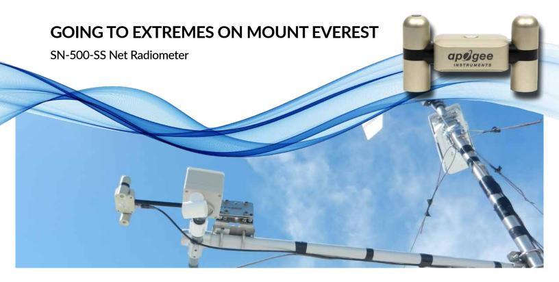
An ambitious multidisciplinary expedition on Mount Everest included an Apogee SN-500 net radiometer to improve weather monitoring in the Khumbu region. A critical part of the network was making sure the automatic weather stations could 1) cope with the extreme conditions of the region 2) minimize their weight for quick and easy installations. The research was published in the Bulletin of the American Meteorological Society in November 2020.
