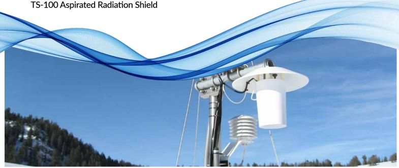
The TS-100 has been deployed for three years on a weather station at a recordsetting cold location in the contiguous United States - Peter Sinks, Utah with the same fan running continuously. It is used to accurately measure the extremely cold air temperatures that occur at the site. The Peter Sinks site uses two yellow-bead thermistors and two PRTs in an Apogee TS-100 to make replicate measurements. Note the Apogee SP-230 all-season pyranometer in the picture as well.
