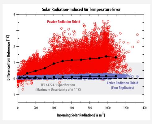
Solar radiation-induced temperature error of Apogee's Class A PRTs (model ST-150) in active shields (Apogee model TS-100) and a passive shield (RM Young six plate) installed on a typical high-reflectance, white-membrane commercial rooftop.
