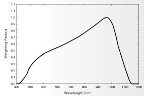
Spectral response estimate of Apogee silicon-cell pyranometers. Spectral response was estimated by multiplying the spectral response of the photodiode, diffuser, and adhesive. Spectral response measurements of diffuser and adhesive were made with a spectrometer, and spectral response data for the photodiode were obtained from the manufacturer.
