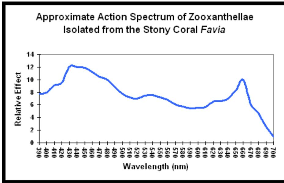
Although quantum sensors are the lowest cost devices for estimating photosynthetic radiation in symbiotic algae in coral, an ideal quantum sensor (exact cutoffs at 400 and 700 nm, equal sensitivity between 400 and 700 nm) may poorly represent photosynthetic radiation because they are designed to equally weight all of the photons between 400 and 700 nm. A waterproof spectroradiometer is an elegant solution to this problem.
