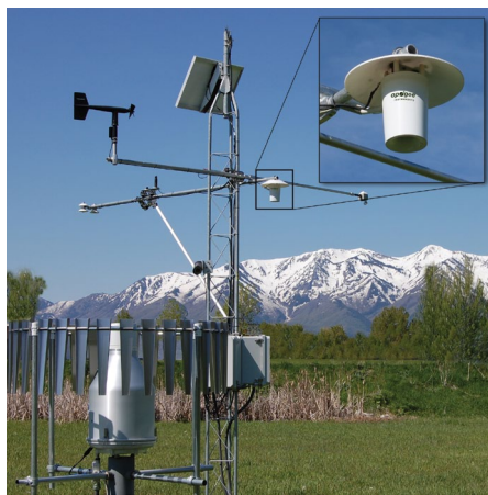
Figure 4: A GAMUT network weather station next to the Logan River in Logan, Utah
